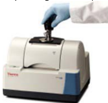
Figure 6.14: Nicolet iS5 FTIR Spectrometer with the ID7 ATR Accessory in the Sample Compartment
