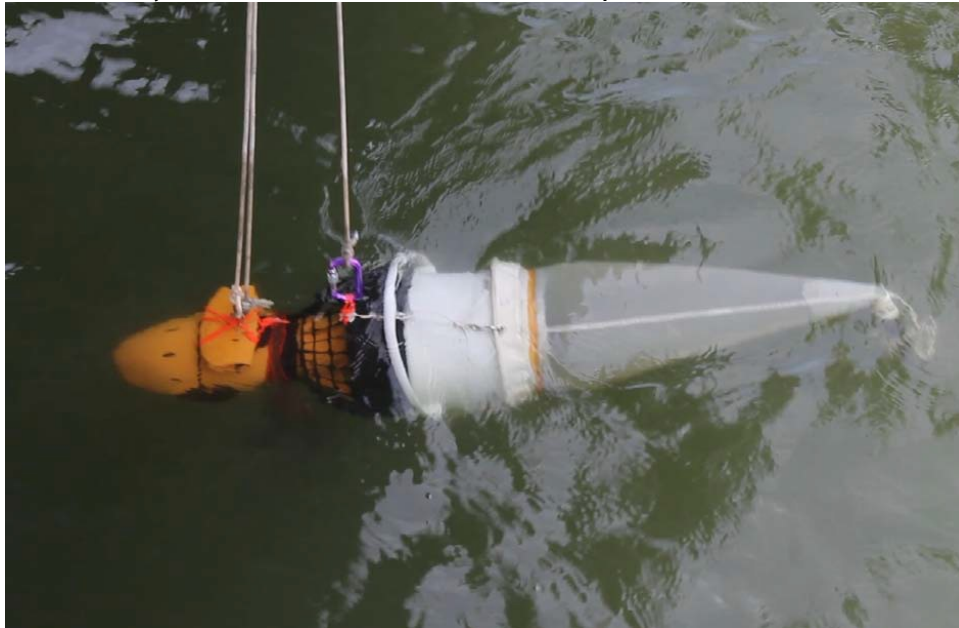
Figure 6.7: Schematic and plate of Microplastics sampling device by Pirika
