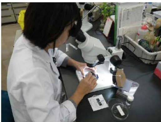
Figure 6.11: Separating Microplastics by Picking and Using the Stereomicroscope (CMSM, 2018) Density
